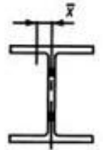
Treat half the flange and portion of web as an angle
