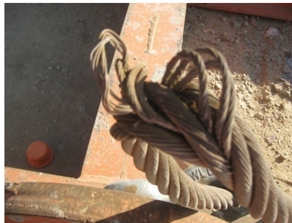
Internal corrosion whilst external surface shows little evidence of deterioration
