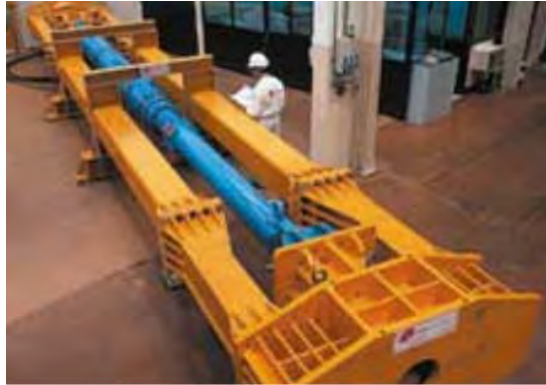
FVDs for the Rion-Antirion Bridge (Greece) under testing at FIP laboratory.
