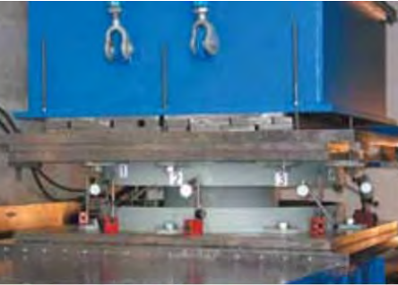
A DCCSS under testing at the Eucentre Laboratory, Pavia, Italy.
