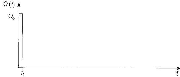
Figure B.13 Dirac pulse loading.
