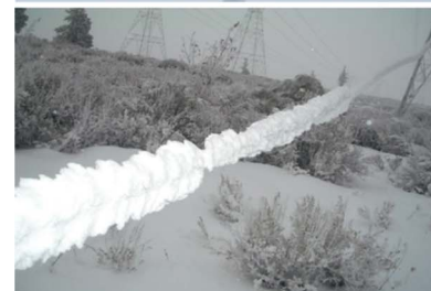
Figure C10.2-2. Rime ice accretion caused by in-cloud icing.
