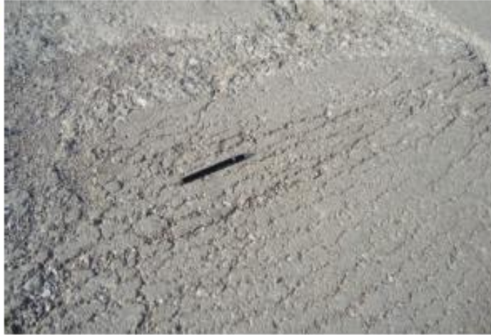
Figure 4.7 Improper moisture content:
