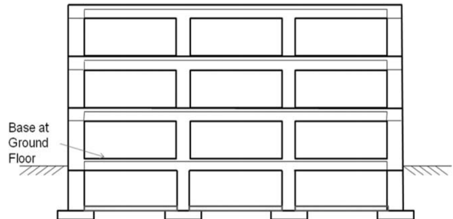
FIGURE C11-3 Base at Ground Floor Level.
