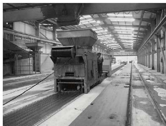
Long line slip form of prestressed hollow core floor slabs, at Bison Manufacturing, United Kingdom.
