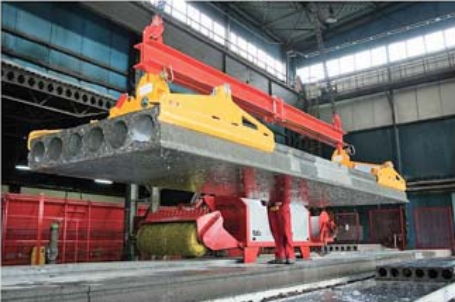
Figure 10.17(a) "Scissors" clamps used for lifting hollow-core floor units both on site and in the factory some 16 hours after casting (courtesy of Spiroll Precast Services Ltd, UK).
