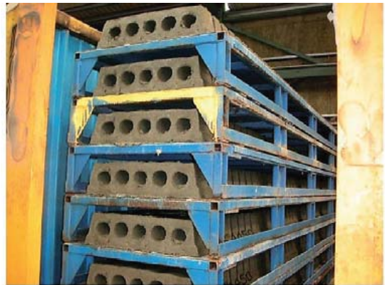
Figure 5.53 After turning over, steam curing of reinforced hollow-core slabs. Manufactured by Creagh Concrete, N. Ireland.
