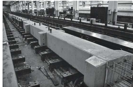
Manufacture of (lightly) prestressed concrete column.
