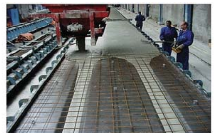
Figure 5.58 Self-compacting concrete grade C50/60 is often used for wet-casting double-tee slabs (courtesy of EFNARC).
